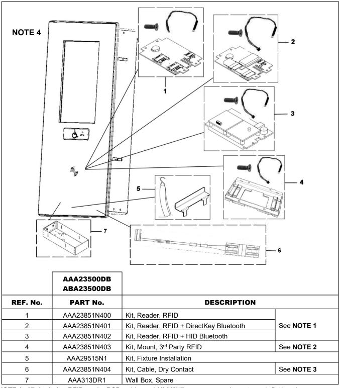
NOTE 1: Kit includes RFID reader PCB, cable, and (4) M2X5 cross recessed countersunk flat head screws.
