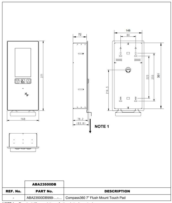
**NOTE 1**: Required 10 mm minimum for bracket release tool.
